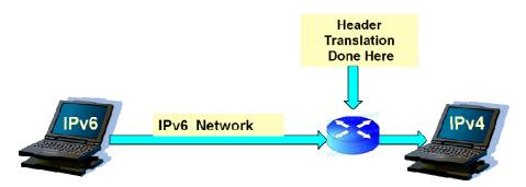
Header translation can be used when sending IPv6 traffic to an IPv4 network as the end destination.
