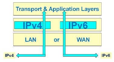
Dual stack can be used when a network handles both kinds of traffic. Virtually all
