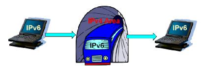
Tunneling is the most precarious method for today's IPv4 networks. The IPv6 packet is included inside the message field of an IPv4 packet. The contents of the IPv6 packet will not be noticed by an IPv4 firewall or intrusion detection system. Cyberterrorists can use this vulnerability to deliver malware, penetrate databases, plant bots, etc.
